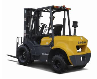
Drive axle is equipped with wide-base and deep tread tires.
