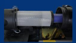
Dual air filter to adapt to dust conditions, prolong the service life of the engine.
